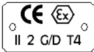
Figure 1: Typical ATEX pump nameplate
